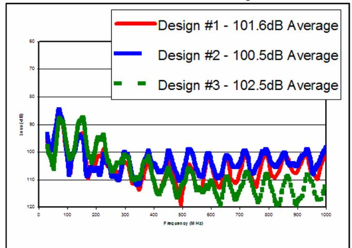
**Figure 4 – Shielding Performance of Low Braid Designs**
