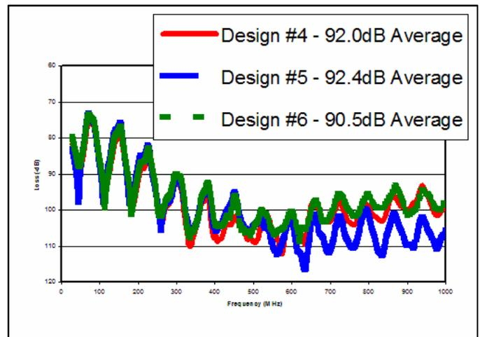
**Figure 5 – Shielding Performance of High Braid Designs**
