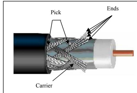
**Figure 1 - Typical Braid Construction**
