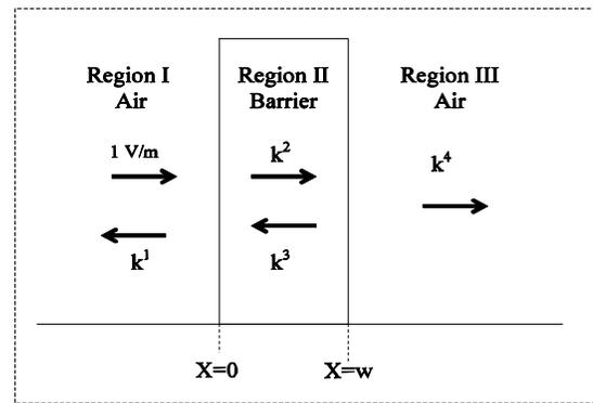
Figure 2. Nomenclature of wave penetrating a barrier
