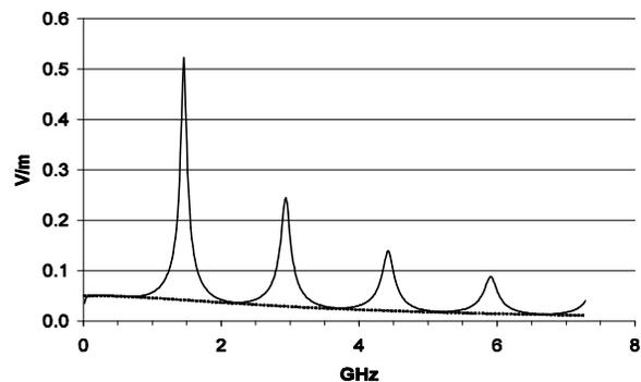
Figure 4. Resonances with resistivity of 20 mhos/m
